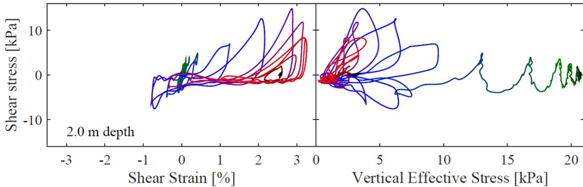
Figure 7: Estimates of the shear stress-strain and effective stress paths of the LEAP 2015 GWU test conducted at Rensselaer.
