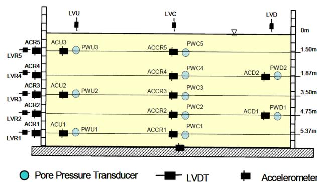
Figure 1: Schematic of a NEES level ground centrifuge test conducted using a laminar box.
