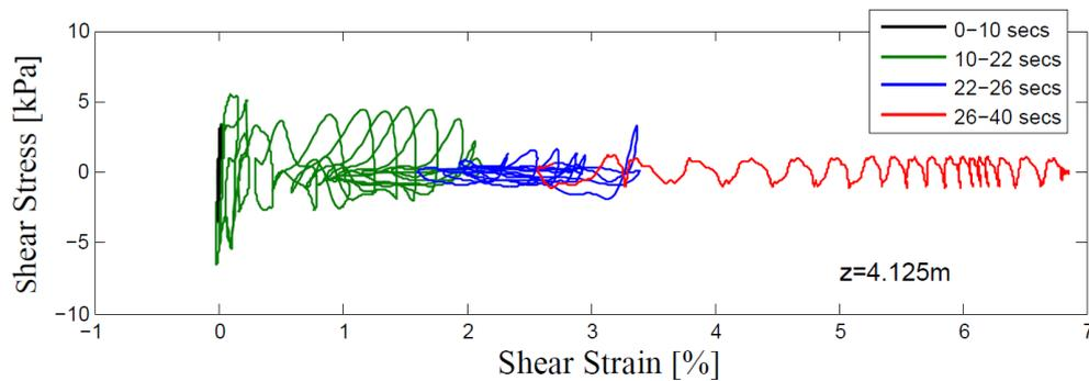
Figure 3: Shear stress-strain response (at about 4.1 m depth) of the model of Figure 1.
