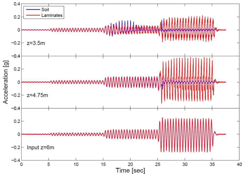
Figure 2: Input acceleration and accelerations recorded at 3.5m and 4.75 m depth of the model of Figure 1.
