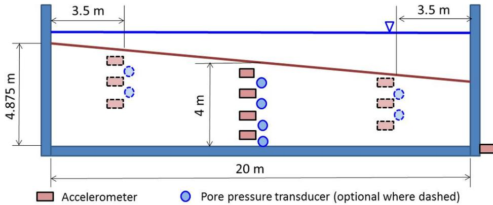
Figure 4: Schematic of the centrifuge model of the LEAP 2015 GWU showing a sloping deposit tested using a rigid box (all dimensions are in prototype units).
