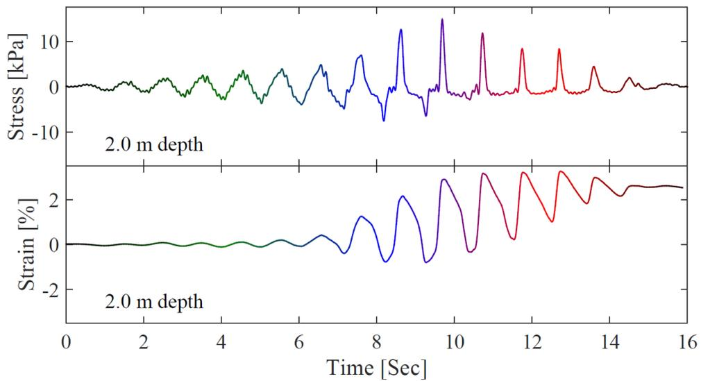
Figure 6: Estimates of the shear stress and strain time histories of the LEAP 2015 GWU test conducted at Rensselaer.
