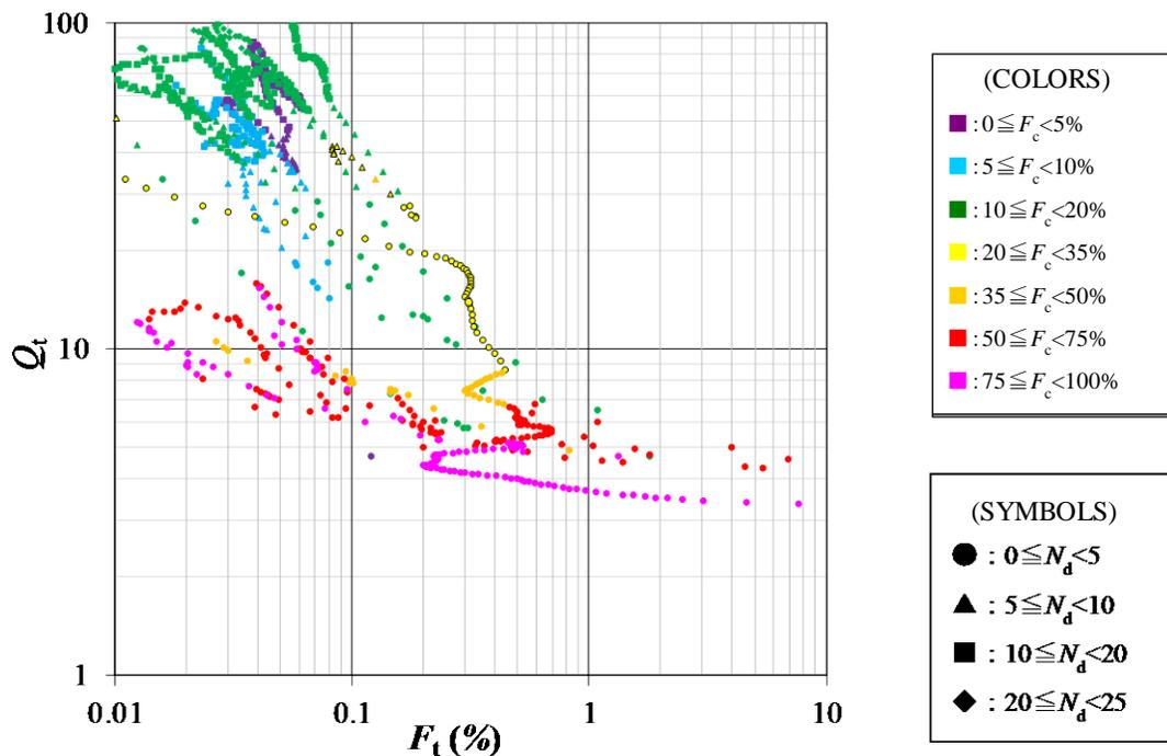
Figure 6. Example for soil classification chart based on PPT
