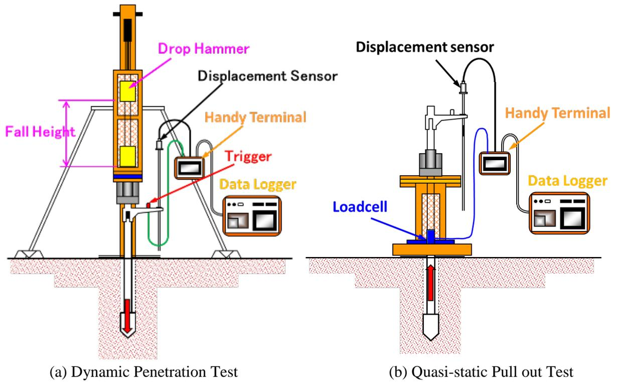
Figure 1. Penetration & Pull-out Test (PPT)
