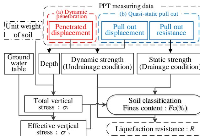
Figure 4. Flow chart of evaluating liquefaction strength using PPT
