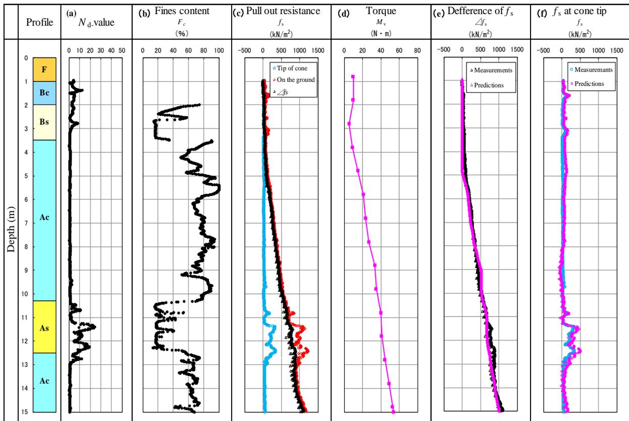
Figure 7. Example of Soil profile and results of PPT
