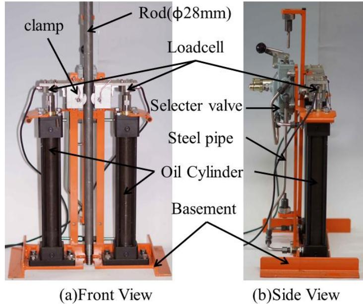
Figure 3. Newly developed pull out equipment
