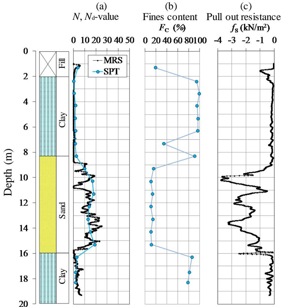
Figure 5. Soil profile by SPT and pull-out resistance
