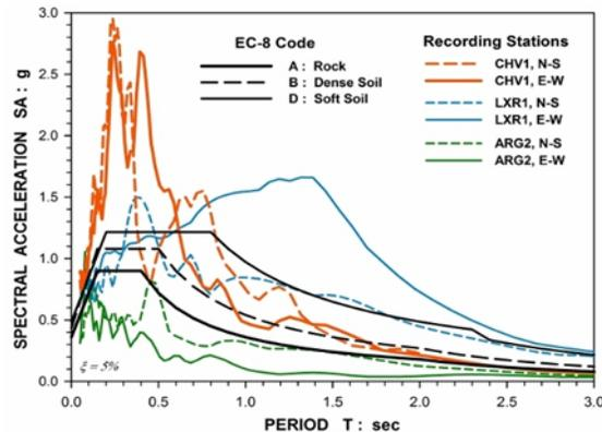
Figure 2. Acceleration spectra from the 2<sup>nd</sup> event, compared to elastic code (EC-8) spectra.
