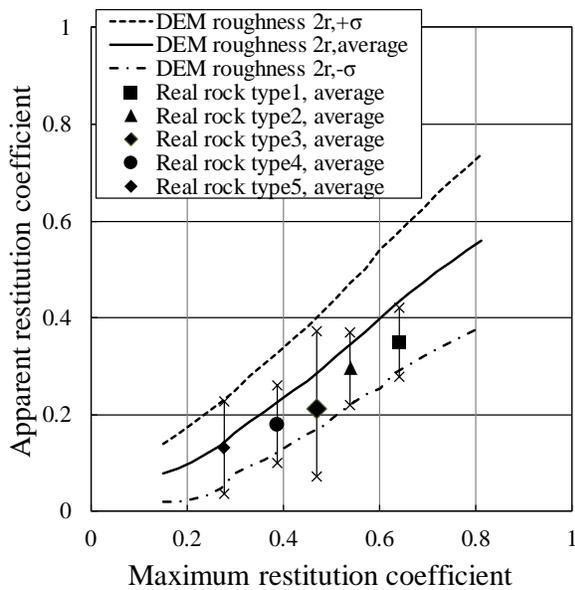
Figure 4. The relationship between maximum restitution coefficient and apparent restitution coefficient
