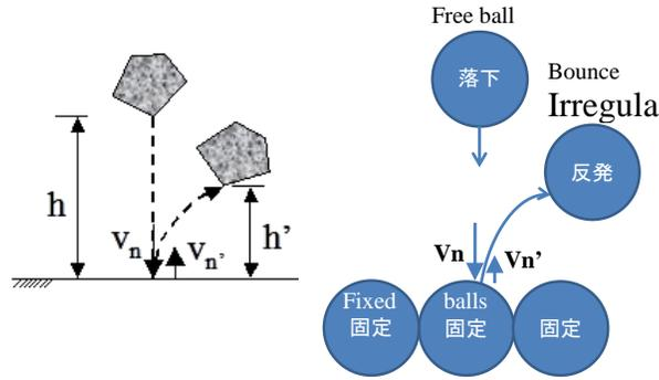
Figure 3. Irregular bounces of a real rock mass and expression by the impact in spherical surface and bounce irregularly
