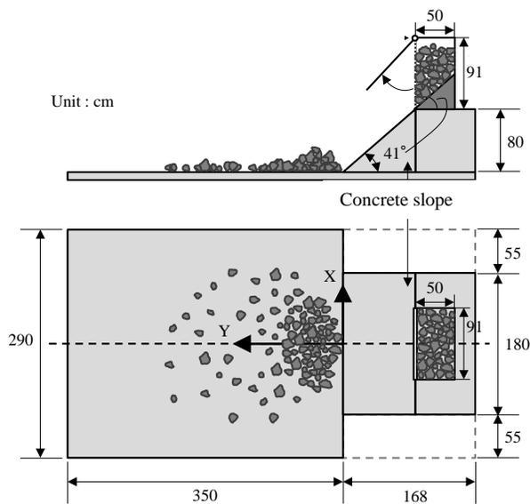
Figure 9. Experiment apparatus.
