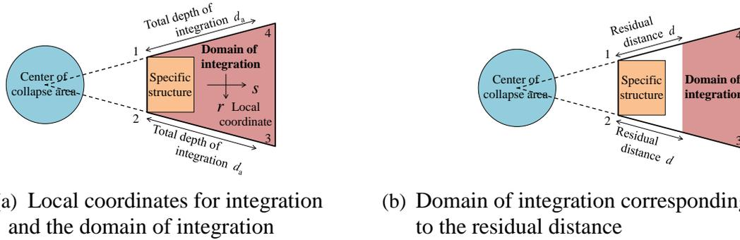
Figure 6. Domain of integration regarding the arrival position coordinates for calculating the collision probability
