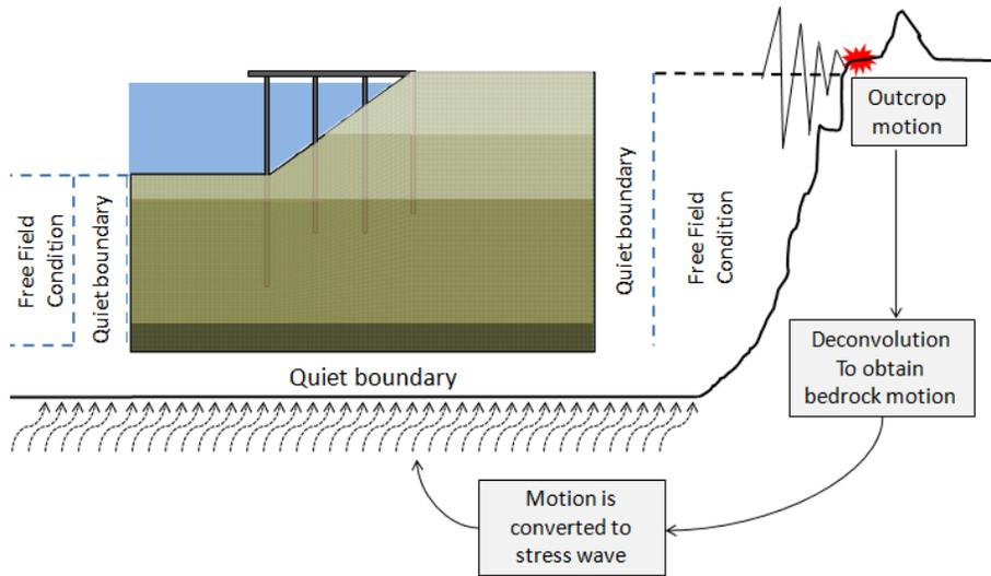
Figure 3. Schematic representation of wharf model, boundary conditions and seismic wave propagation implemented in FLAC.
