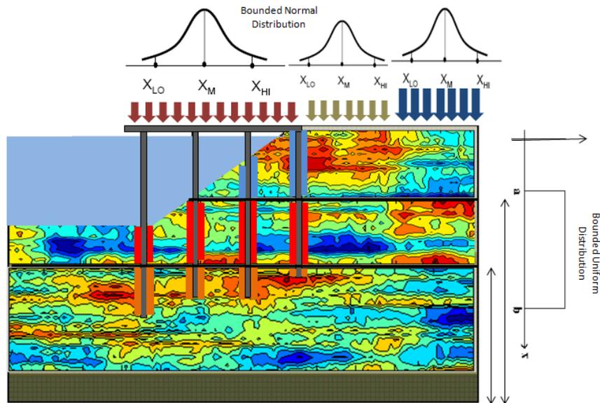
Figure 7. Stochastic representation of soil properties, layering pattern and loads on deck and backland.
