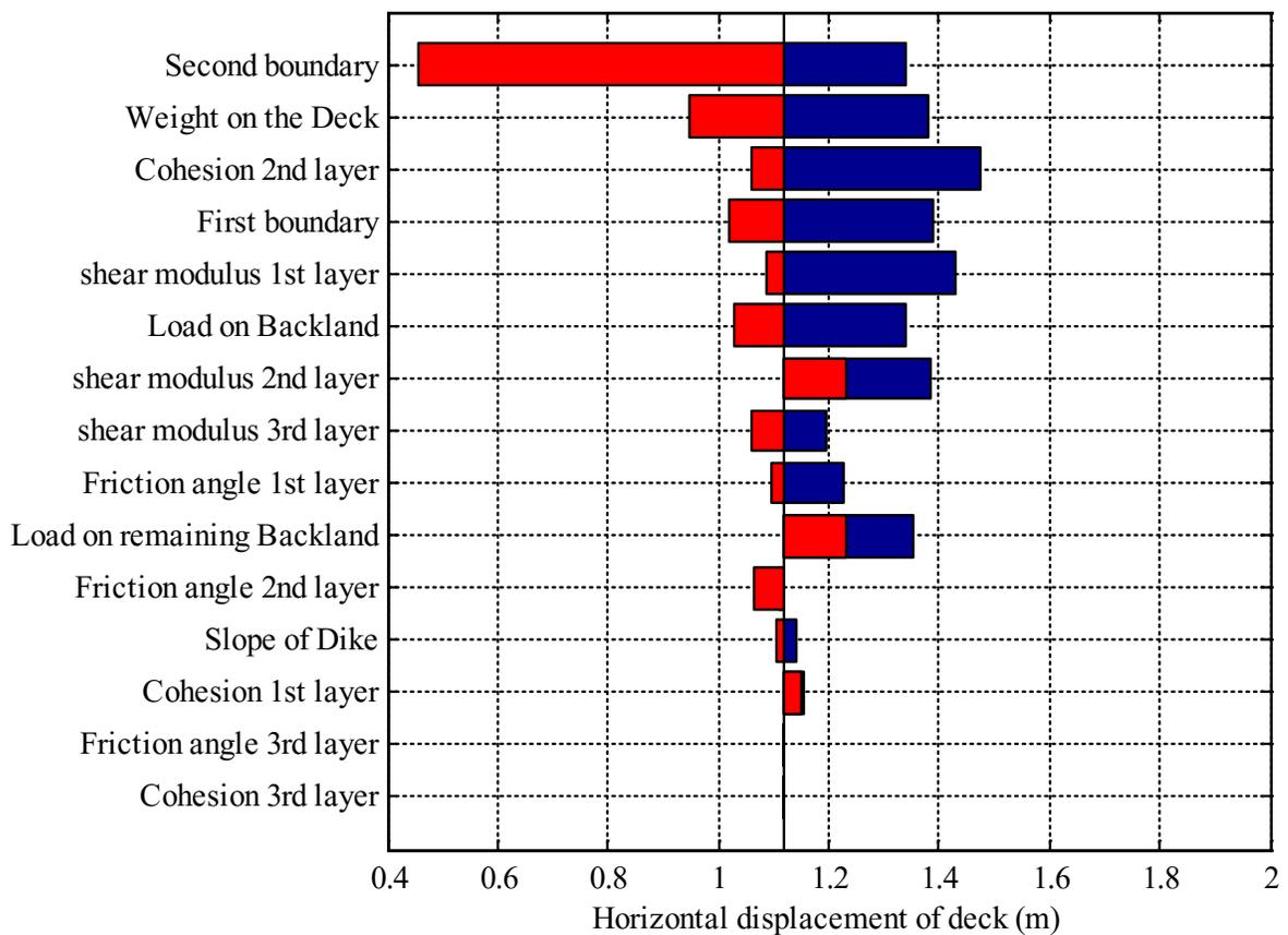
Figure 5. Results of Tornado sensitivity analysis, showing sensitivity of residual displacement of the deck to different variable specifications of the wharf.
