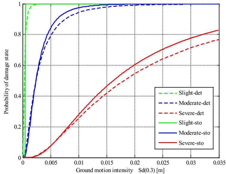
Figure 8. Comparison of fragility curves obtained from deterministic and stochastic model of the target wharf
