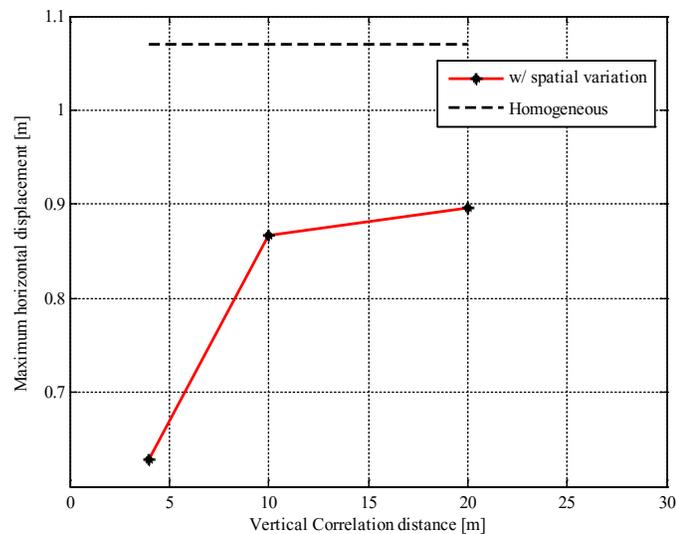
Figure 6. Comparison of displacement of deck with homogenous and spatial variation in vertical direction with random fields assuming vertical correlation distances of 4, 10 and 20m.
