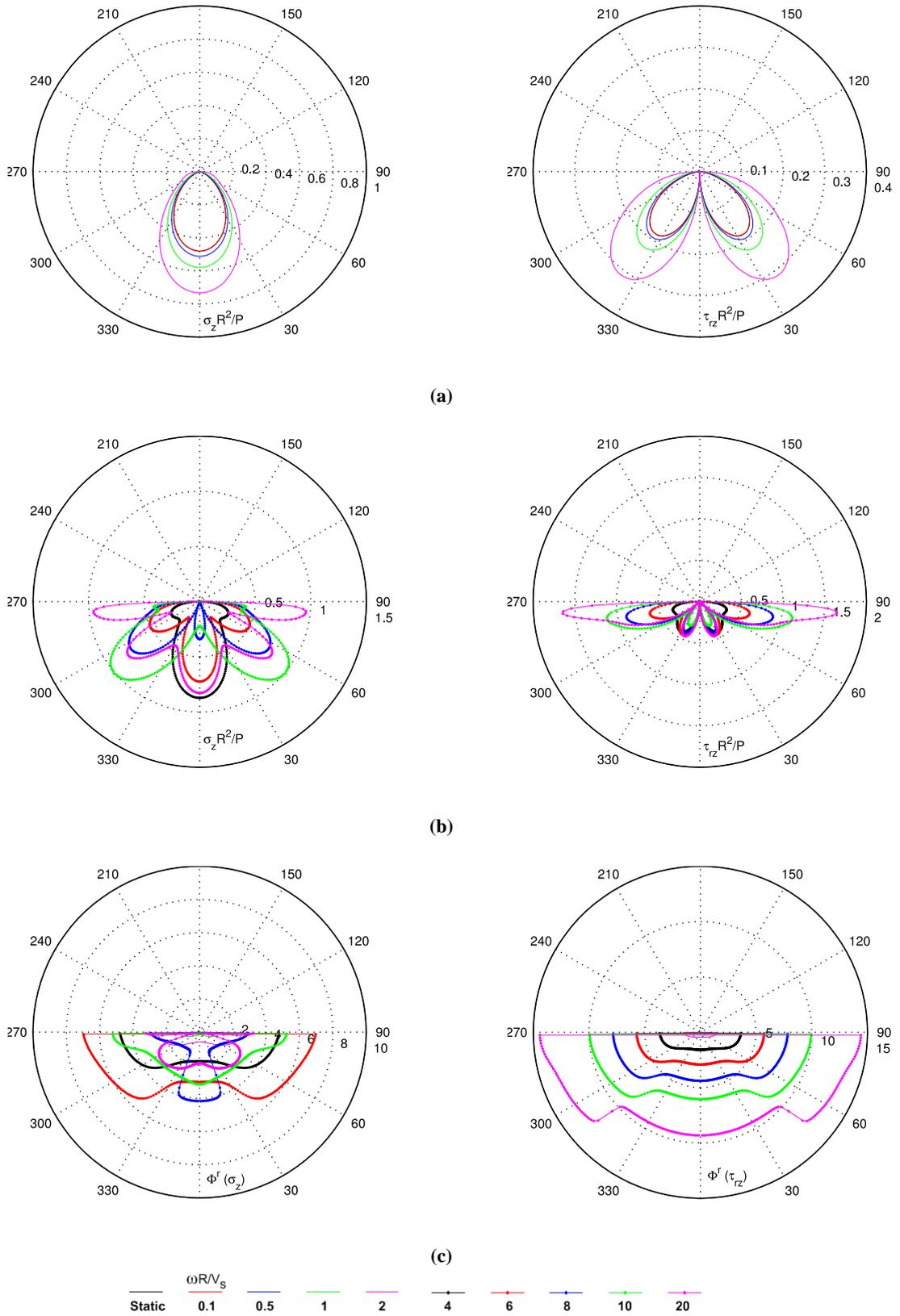
Figure 4. Stress bulbs due to vertical point load,  $\nu = 0.34$ ,  $\zeta = 5\%$ ; (a) Stress amplitude bulbs for  $\omega R/V_s = 0$  (static) to 2, (b) Stress amplitude bulbs for  $\omega R/V_s = 4$  to 20, and (c) phase angle bulbs for  $\omega R/V_s = 0$  to 20.
