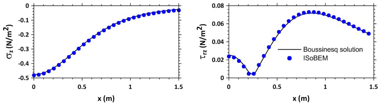
Figure 2. Comparison between ISoBEM and analytical solution for classical Boussinesq problem ( $y = 0$ ,  $z = -1$  m,  $P = 1$  N,  $\rho = 1.8$  Mg/m<sup>3</sup>,  $V_s = 100$  m/s,  $\nu = 0.33$ )
