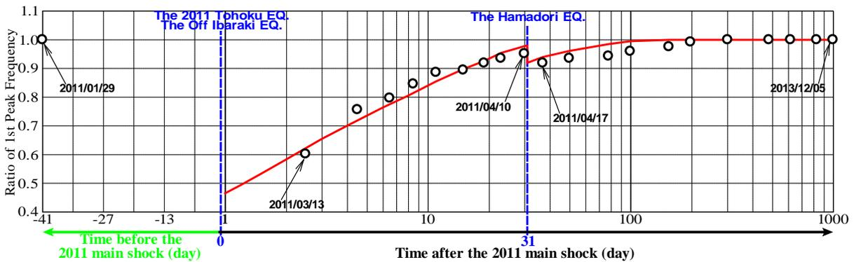
Figure 3. Peak frequency of observed and simulated microtremor H/V spectra
