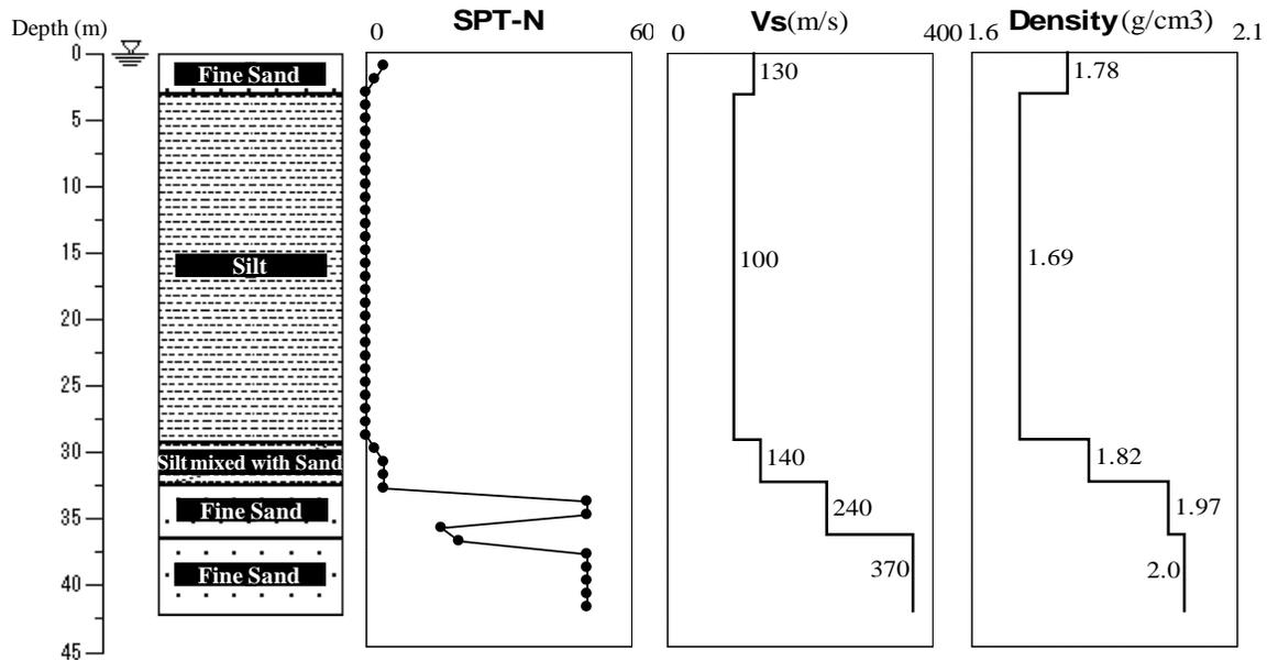
Figure 1. Soil profile from engineering bedrock to ground surface at the site of interest
