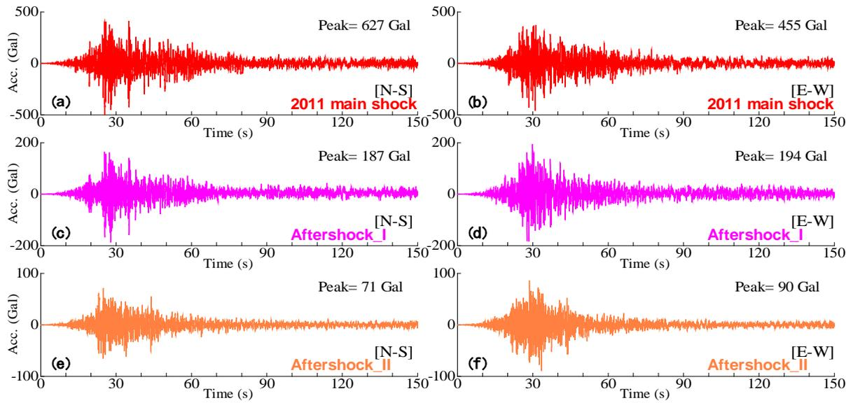
Figure 5. Input earthquake motion
