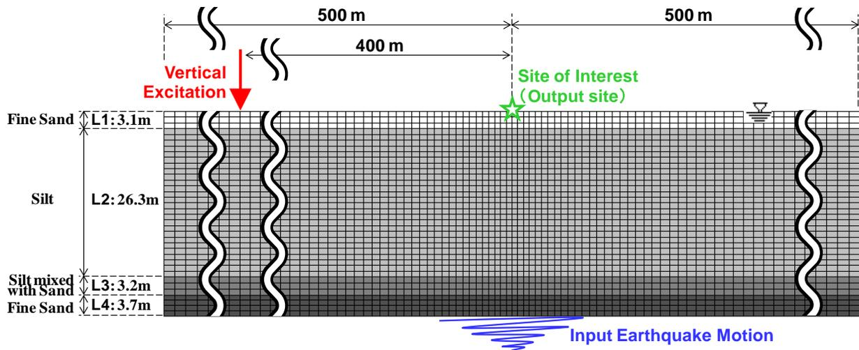
Figure 4. Dynamic FEM model for microtremor and earthquake motion
