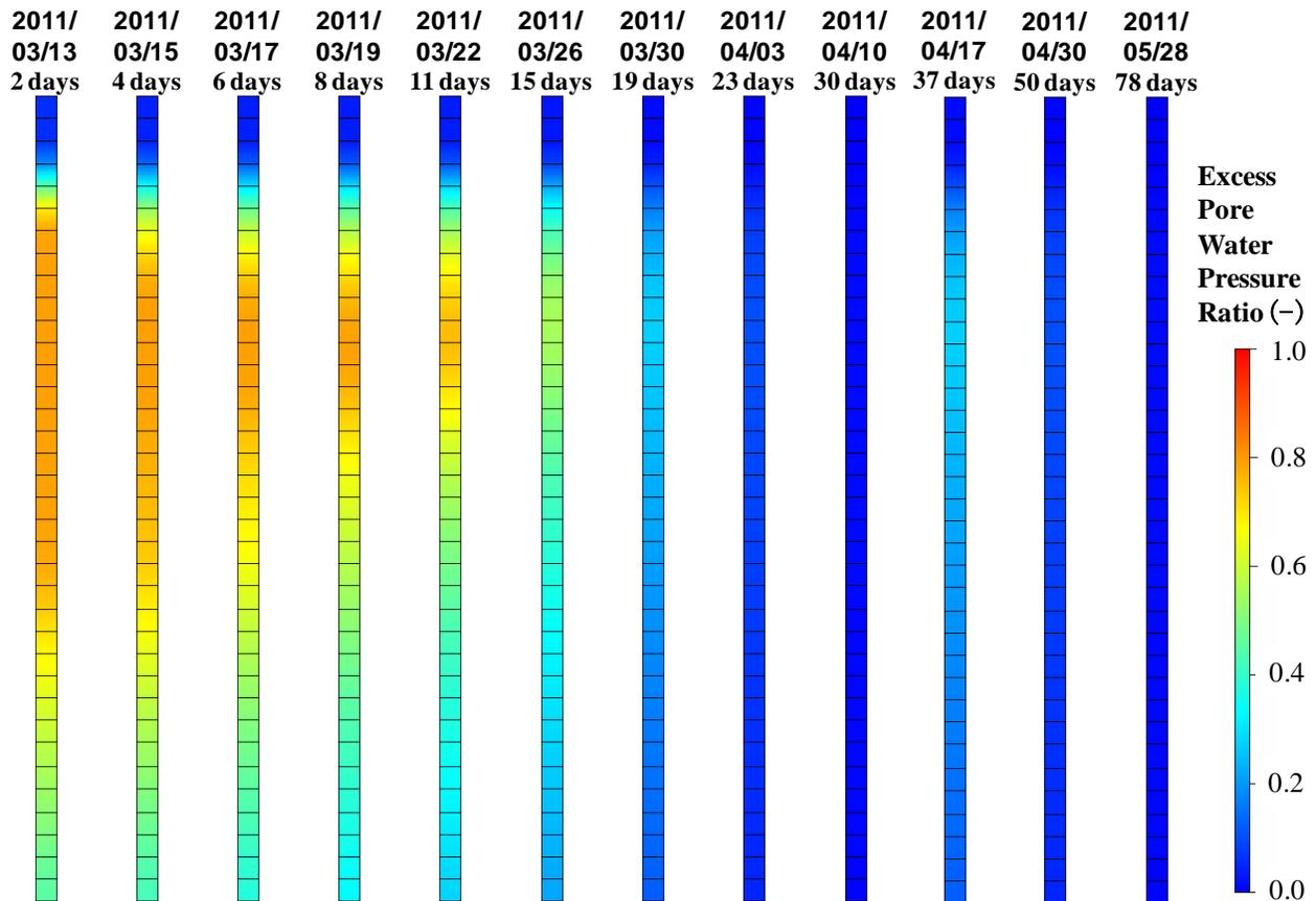
Figure 6. Distribution of excess pore water pressure ratio based on the effective stress analysis
