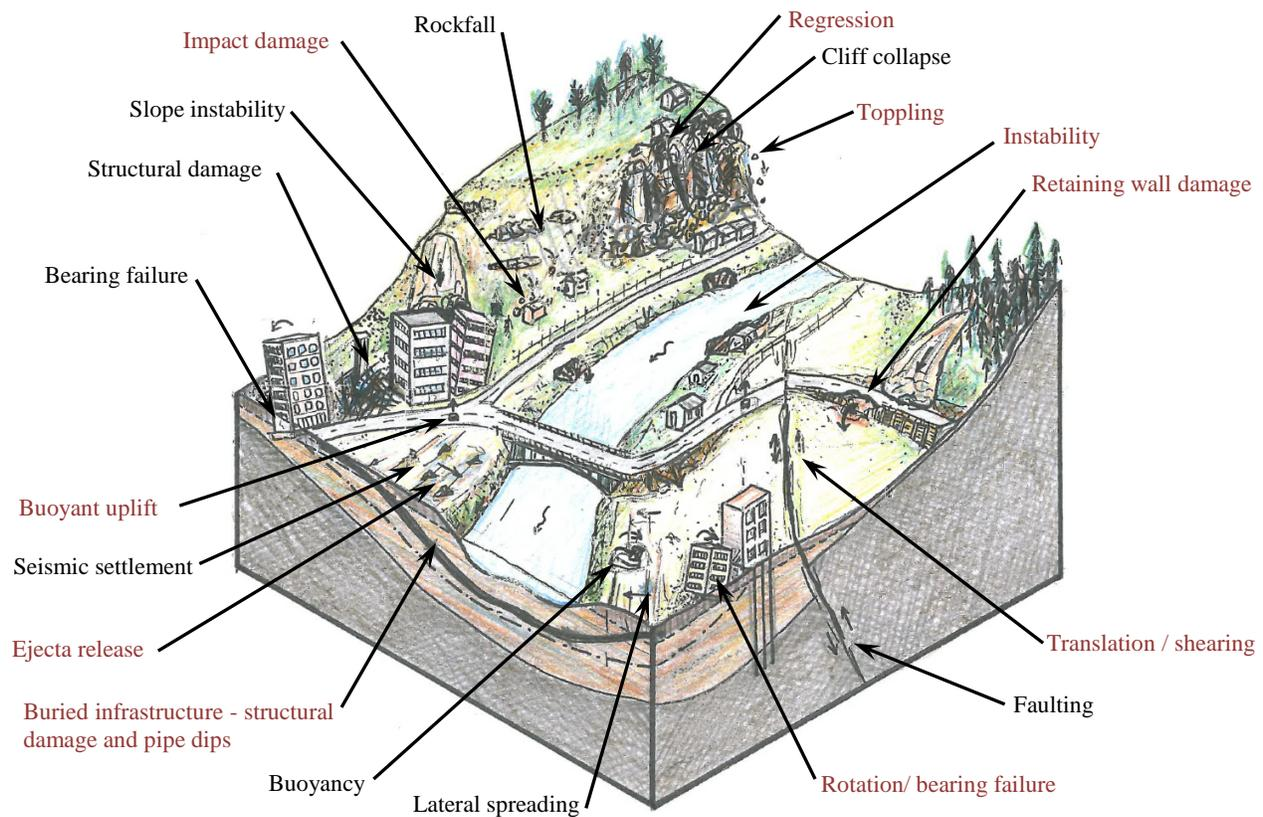
Figure 3. Schematic representation of typical geological and geotechnical hazards
