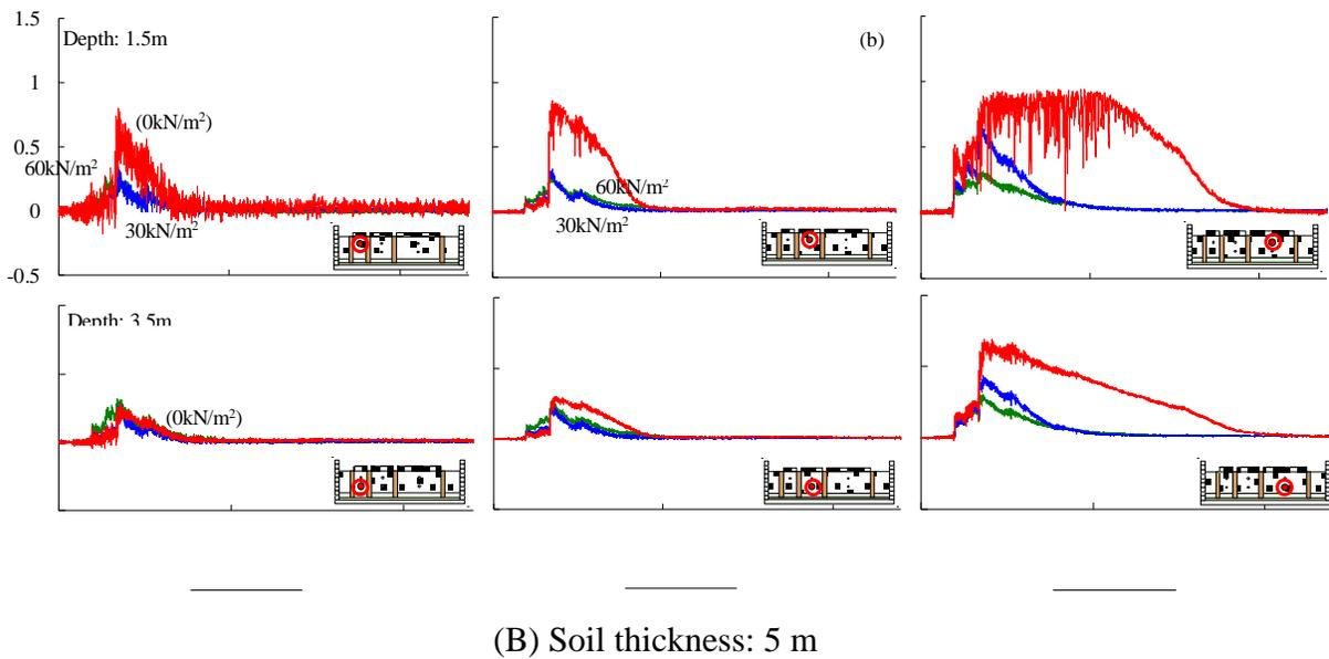
Figure 4. Excess pore water pressure ratio observed in the centrifuge tests
