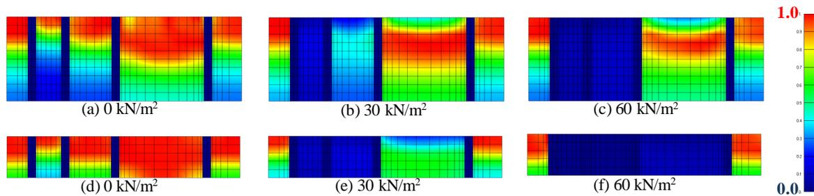
Figure 8. Contour of excess pore water pressure ratio
