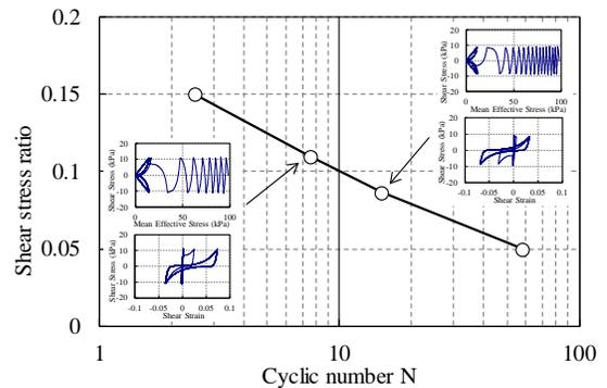
Figure 6. Model parameters and liquefaction strength of the constitutive model
