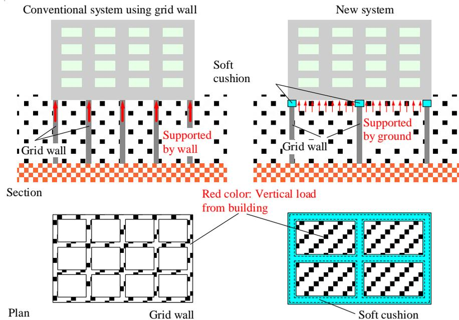
Figure 1. Conventional countermeasure and proposed new system
