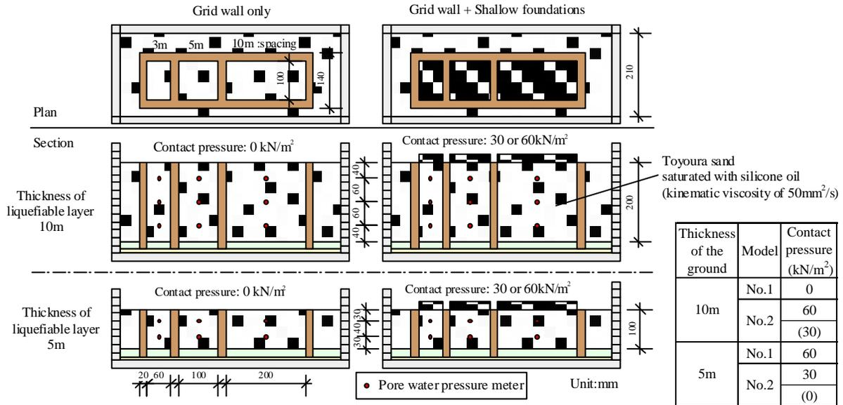
Figure 2. Physical models for centrifuge testing
