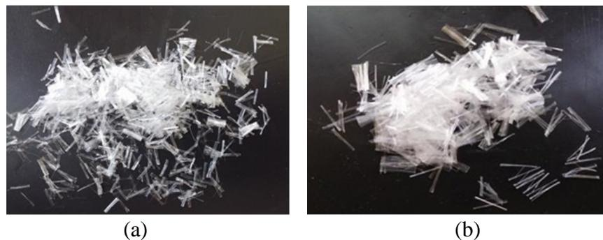
Figure 1. Materials used in this study (a) 6 mm PP fibers, and (b) 12 mm PP fibers
