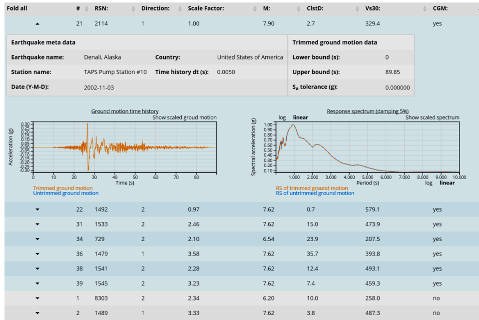
Figure 4. CGMapp user interface showing the first characteristic ground motion from the list of selected hazard-consistent ground motions
