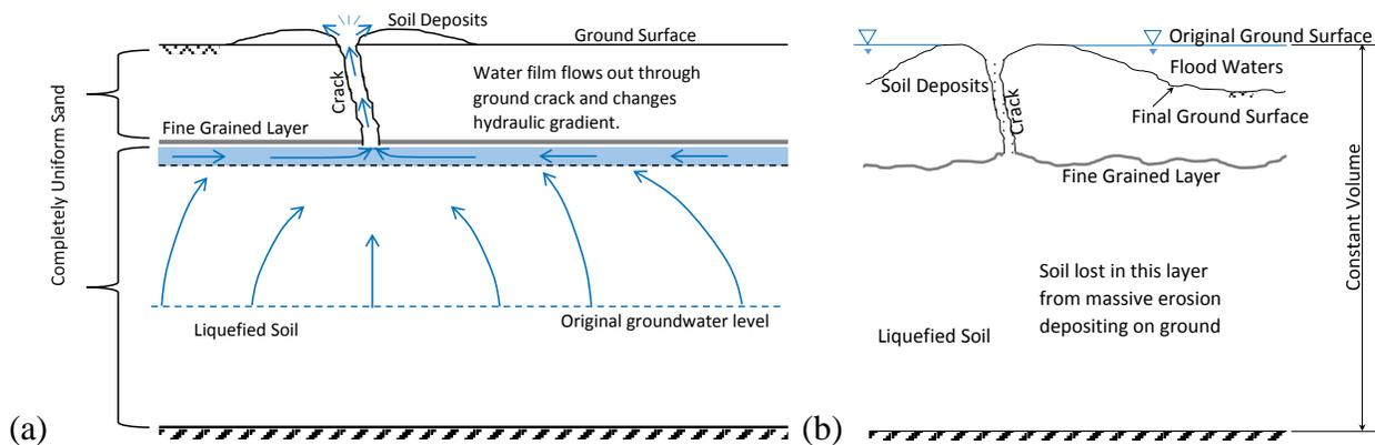
Figure 3. Continuous fine grained layer within otherwise uniform sand. (a) Upward water flow slowed at fine grained layer forming a water film; crack focuses soil-water slurry ejection on ground surface and changes hydraulic gradient. (b) Final state of uneven ground conditions.
