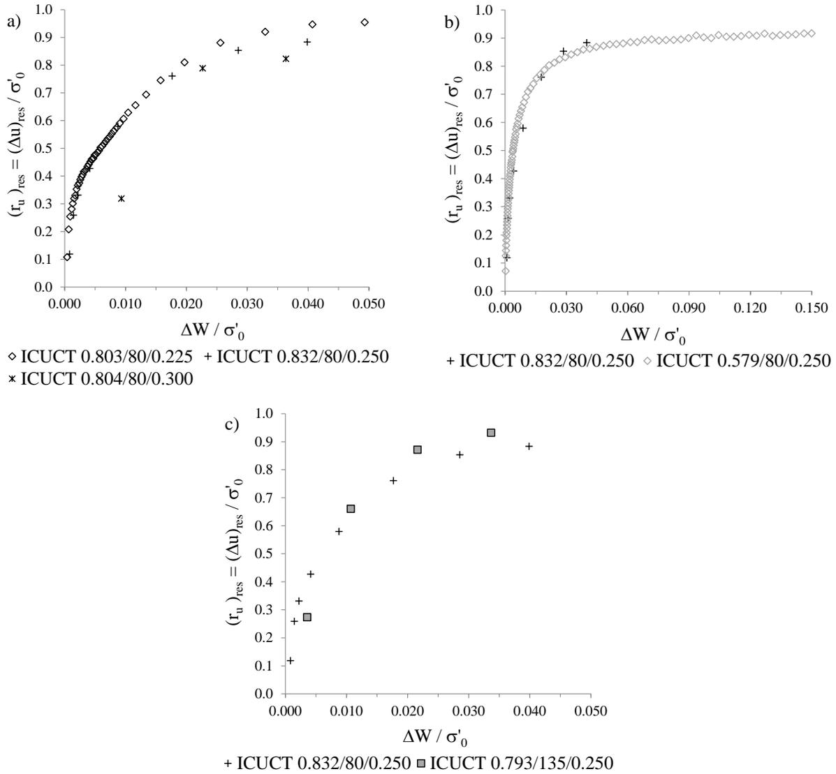
Figure 3. Influence of (a) CSR, (b)  $e_0$  and (c)  $\sigma'_0$  on the relationship between residual excess pore water pressure ratio build-up and normalised dissipated energy per unit volume
