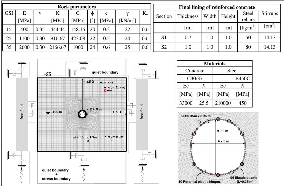
Figure 2: Numerical model and parameters used to define fragility curves.
