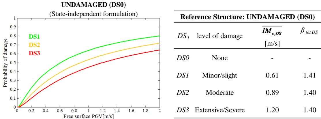
Figure 4: State-independent fragility curves obtained to validate the proposed procedure.
