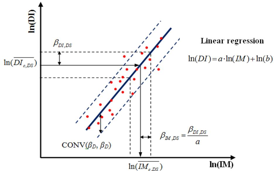
Figure 1: Approach used in this work to define the parameters required to draw the fragility curves.
