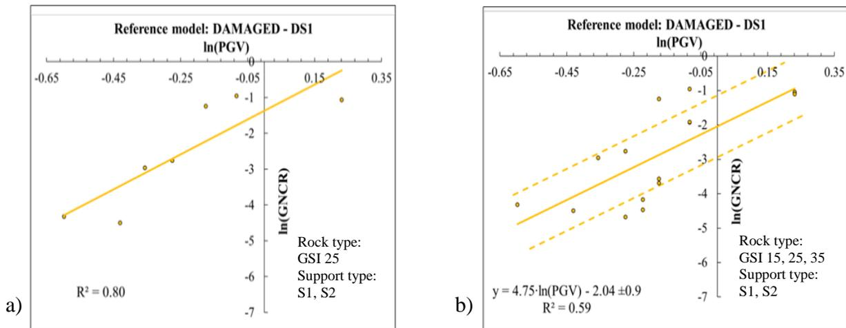
Figure 3: Example of linear fit to define the parameters required to draw the fragility curves (here are reported only data related to a system with an initial level of damage equal to DS1).
