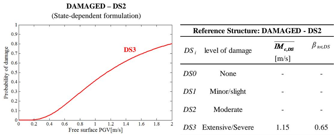
Figure 5: State-dependent fragility curves obtained to validate the proposed procedure.
